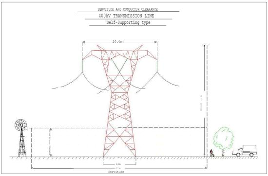
Figure 2-5:Self-supporting Suspension Tower
