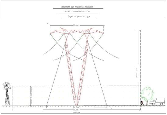
Figure 2 -6: Guyed Suspension Tower
